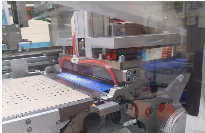
Figure 3.8: String cutting station.
