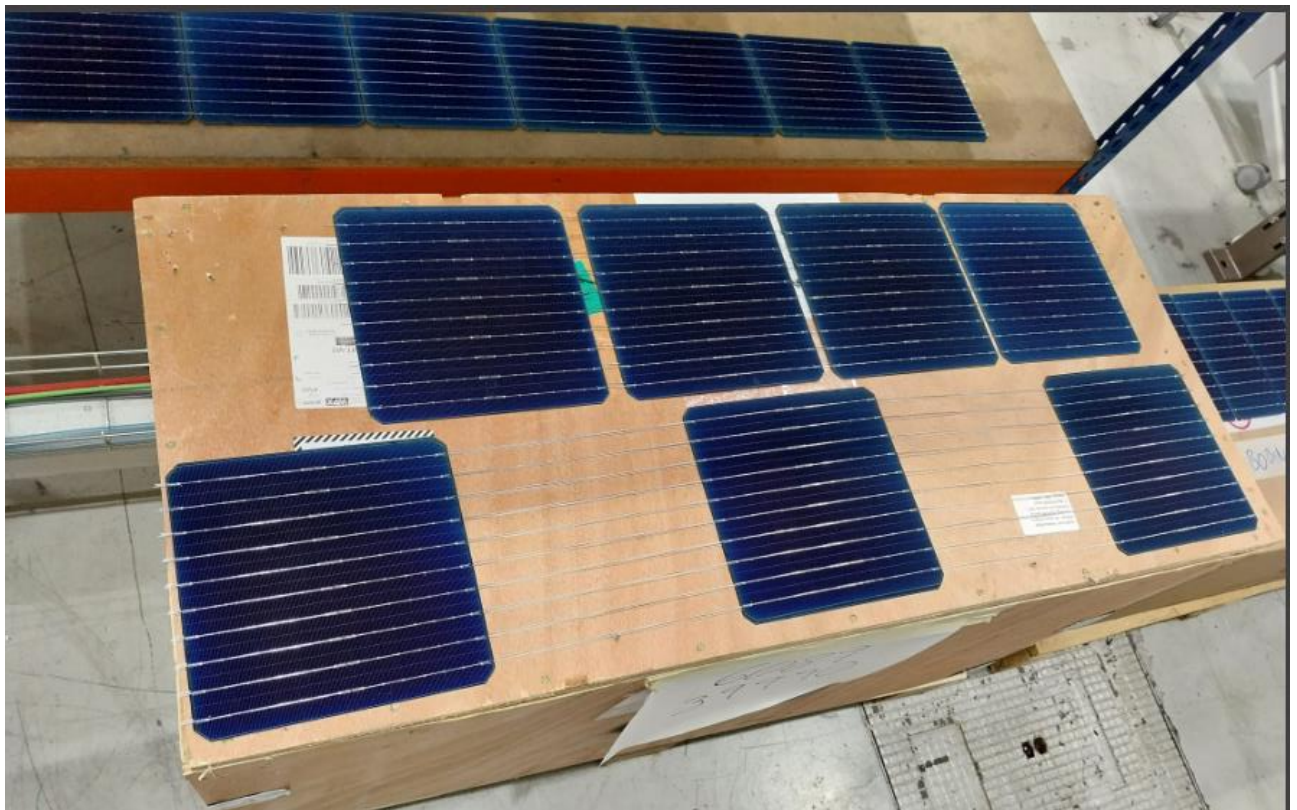
Figure 2.8: String samples, 1x Standard mode+ 2 X BIPV mode.
