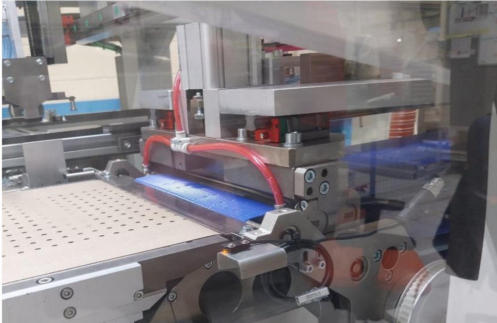
Figure 2.7: String cutting station.
