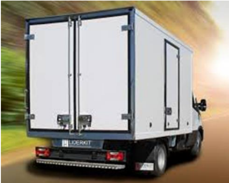
Figure 2.24: Isothermal Cargo Box type (Liderkit)
