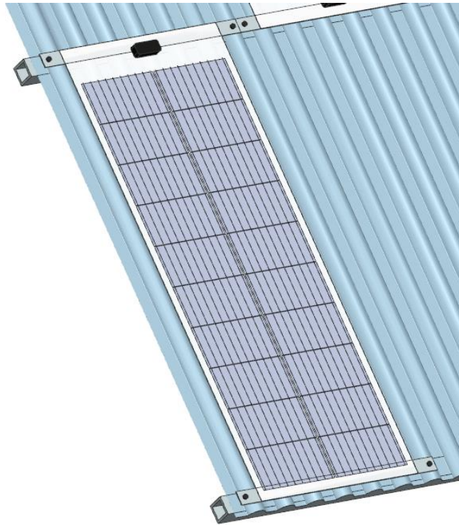
Figure 2.36: Demo 9 - Fixing method of the AgriPV module
