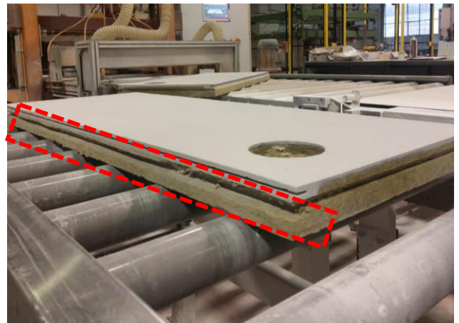
Figure 8. Cutting machine No. 2 in action and output PIZ panel after cutting machines
