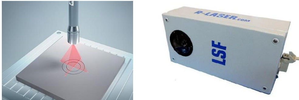
Figure 9. Laser projector for projecting image of cells and JB over PIZ panel
