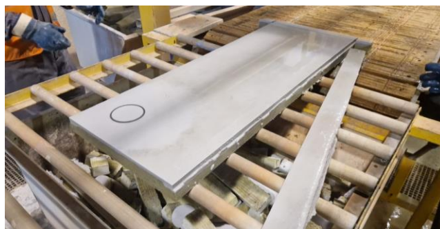
Figure 6. PIZ output PIZ panel from cutting machine
