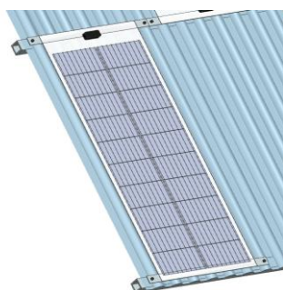
Figure 5-11: Fixing method of the AgriPV module
