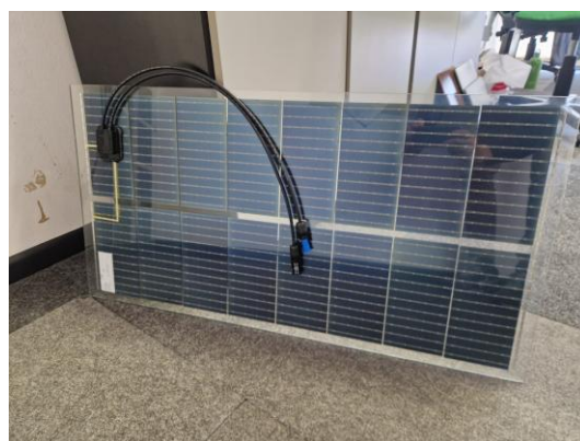
Figure 2-7: 3S PV module (rear view)
