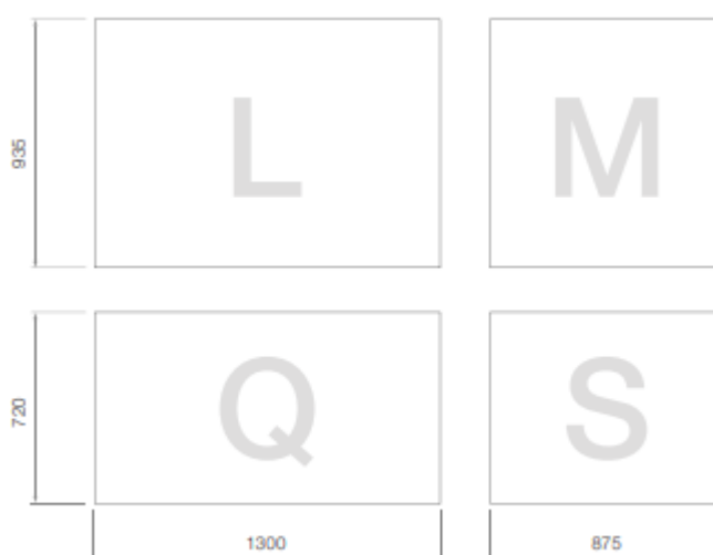
Figure 3-2: Standard dimensions of 3S modules
