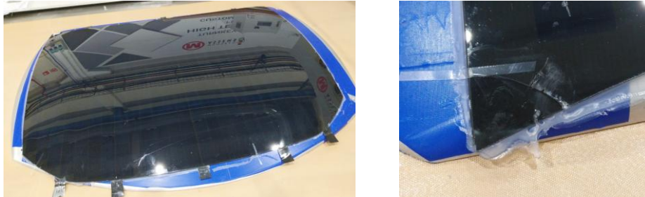
Figure 4.4: The laminated module using Test # 10 processing parameters.
