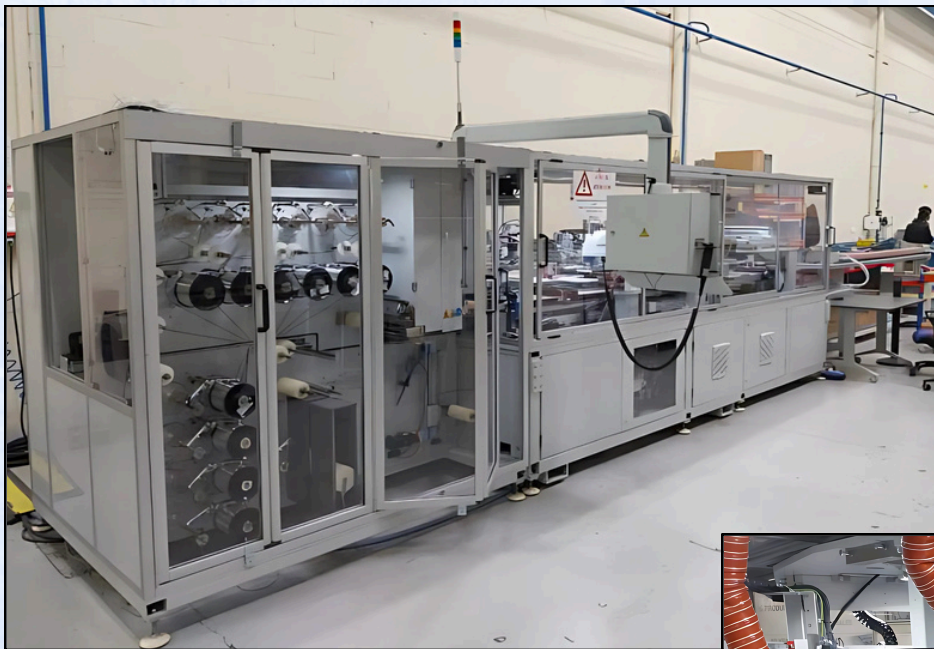
◀ Figure 2: view of the complete tabber-stringer
